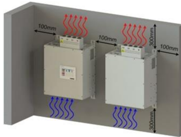
Figure 2: Positioning the AHF Wall Type Device
